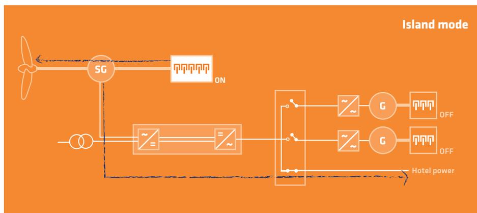
**Island mode** allows the entire electrical network to be created by the drive train to feed all electricity needed by the network. The auxiliary gensets are switched off. The shaft generator and converters take care of all power needed.
