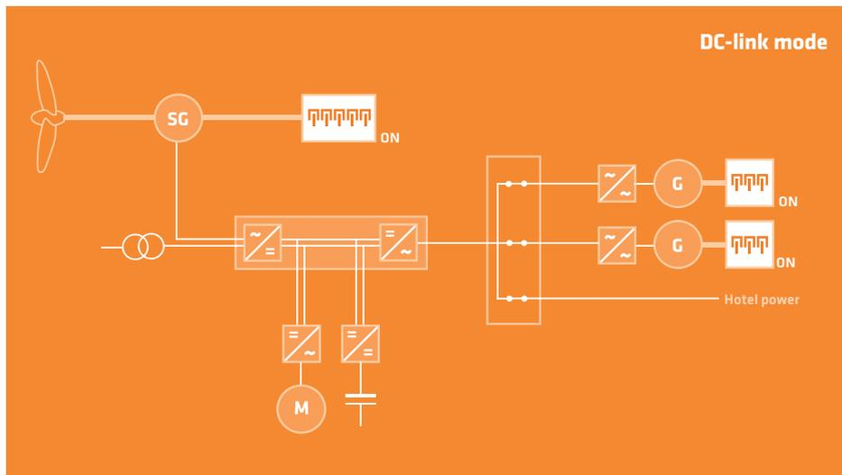
**DC-link** mode: with the inclusion of a DC/DC converter and battery bank, the PTI mode can achieve a really advanced operational optimization. The DC-link creates new possibilities for advanced ship design. The main switchboard can be smaller, and heavy users, such as big pumps, thrusters or battery banks, can be run more efficiently.
