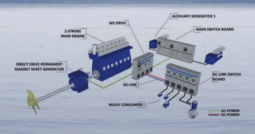
The WE Drive system removes the need for constant speed operation by using variable frequency drive technologies in shaft generator systems
