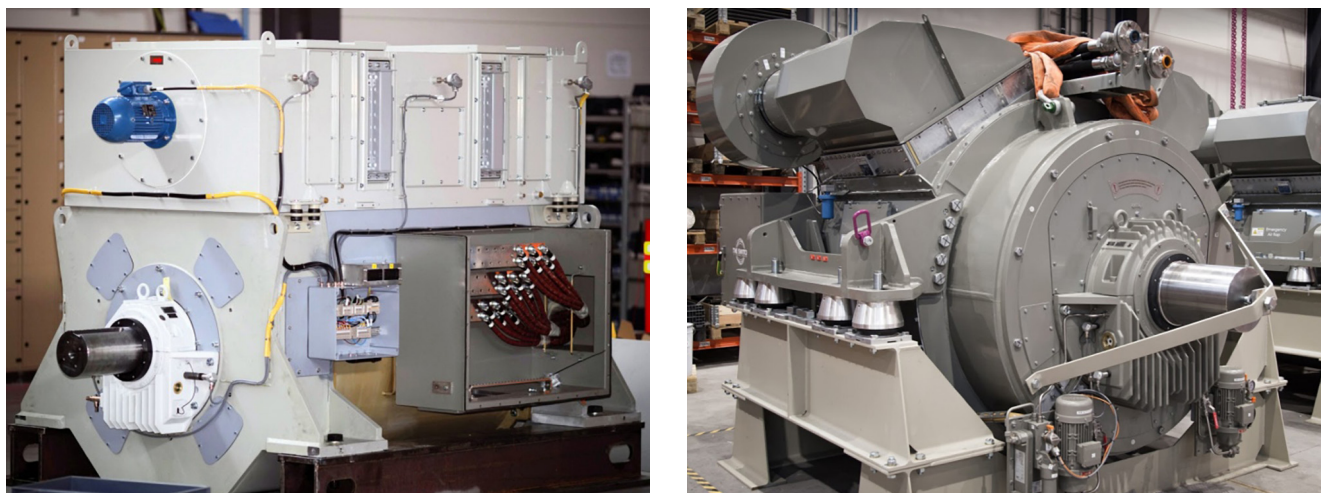
Figure 1: Generator on the left during final assembly and before painting, and the motor on the right.
