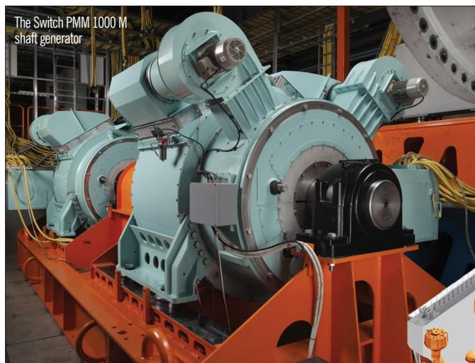
The Switch PMM 1000 M shaft generator
