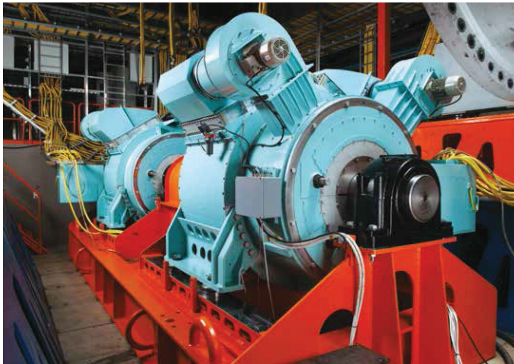
Capable of operating in a speed range from 0-100 rpm, the permanent magnet machine has a constant power of 1.5MW (credit: The Switch)
